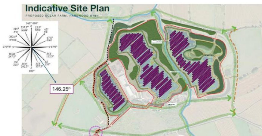
Figure 11: Site plan with solar panel orientation revised to reduce glint and glare
